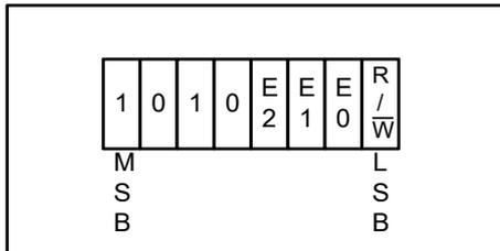
The three E2, E1, and E0 device address bits allow as many as eight devices on the same bus. These bits must compare to their corresponding hardwired input pins.
